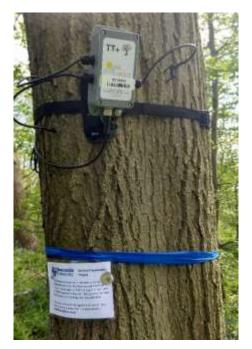
project now has concerns regarding their value. Many sensors have seen their cables and connections failing, mainly due to corrosion.
